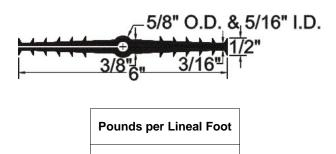
TPER Waterstop is manufactured from a specially formulated Thermoplastic Vulcanizate Rubber. This product has excellent physical properties and chemical resistance and will assure an owner of a facility that require containment for environmentally sensitive materials.
