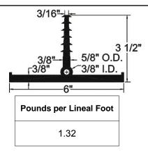
TPER Waterstop is manufactured from a specially formulated Thermoplastic Vulcanizate Rubber. This product has excellent physical properties and chemical resistance and will assure an owner of a facility that require containment for environmentally sensitive materials
