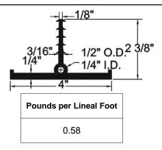
TPER Waterstop is manufactured from a specially formulated Thermoplastic Vulcanizate Rubber. This product has excellent physical properties and chemical resistance and will assure an owner of a facility that require containment for environmentally sensitive materials
