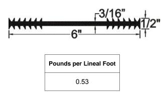
TPER Waterstop is manufactured from a specially formulated Thermoplastic Vulcanizate Rubber. This product has excellent physical properties and chemical resistance and will assure an owner of a facility that require containment for environmentally sensitive materials.
