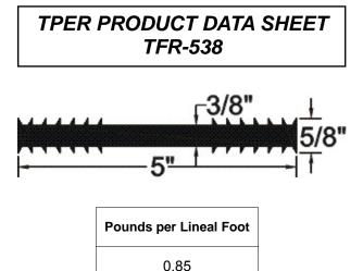
TPER Waterstop is manufactured from a specially formulated Thermoplastic Vulcanizate Rubber. This product has excellent physical properties and chemical resistance and will assure an owner of a facility that require containment for environmentally sensitive materials.
