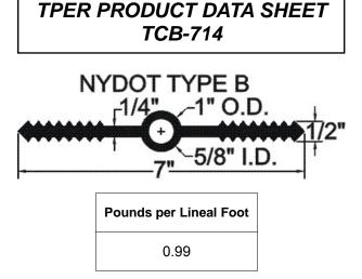
TPER Waterstop is manufactured from a specially formulated Thermoplastic Vulcanizate Rubber. This product has excellent physical properties and chemical resistance and will assure an owner of a facility that require containment for environmentally sensitive materials.
