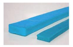
*HydroStrip* Hydrophilic Chloroprene Rubber pre-exposure to water and 400% swell after 30 days exposure in freshwater.
