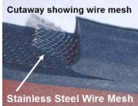
MC-2010MN has excellent durability and resistance to chemical contaminants. It can perform in a wide range of solutions such as seawater or cement water. The material does not contain any toxic substance or heavy metals and is environmentally safe. **MC-2010MN IS NSF 61 CERTIFIED.**
