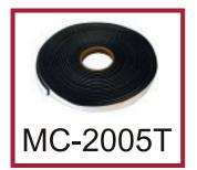
MC-2005T is a 20mm x 5mm (approx. 0.8" x 0.2") chemically modified natural rubber (non-vulcanized) product. The manufacturing process chemically bonds a hydrophilic agent to the rubber. This product is used in concrete joint work where hydrostatic head does not exceed 50 feet. It performs in a wide range of solutions such as seawater or cement water. This material does not contain any toxic substance or heavy metals and is environmentally safe. It comes 320 feet / case.
