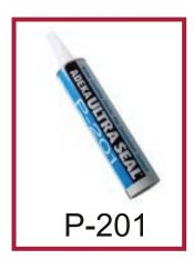
P-201 is a water swelling, single component, elastic sealant which expands up to 2 times by volume (100%). It is used in variety of places such as cold/construction joints, expanded metal forms, piping penetration, etc. P-201 is used as a waterstop in new construction and in repair applications which can be placed on damp or uneven surfaces and functions in a wide range of temperatures and ground water conditions. It comes 24ea- ~11oz cartridges / case or 3.17 gal / pail.
