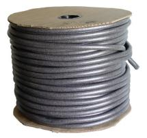
BoMetals Standard Backer Rod (FBR) is a ideal non aborbent compressible polyethylene material inserted into a joint to control sealant depth, creating a backstop to allow proper sealant tooling. It can also be used as a temporary joint seal.
