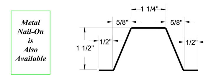
Plastic Nail-On Keyway is nailed to a form prior to pouring Installed in tilt-up work, industrial floors, curbs or wherever specified Simple to use, lightweight and reusable BoMetals quality that you've come to recognize 10-foot lengths – 400' per box
